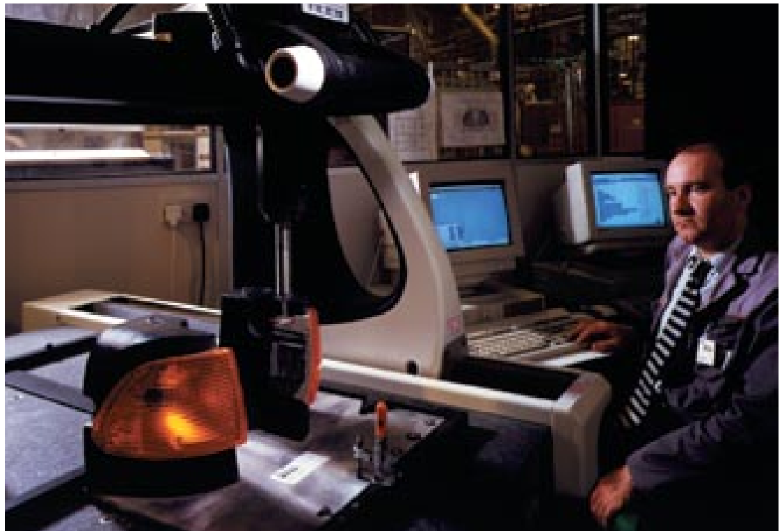
The dimensions of a BMW 7 Series turn signal lens are checked on a DEA SWIFT coordinate measuring machine at Britax Vega Ltd. The move to CMMs has given the company the flexibility it needs to inspect a wide range of products.
