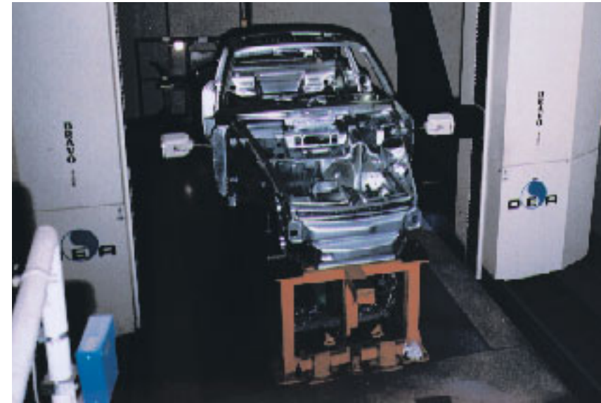
Dual-arm DEA BRAVO measuring robot speeds body-in-white inspection at the Porsche Stuttgart plant. Dimensional data is used to control welding machines in the body assembly operation.
