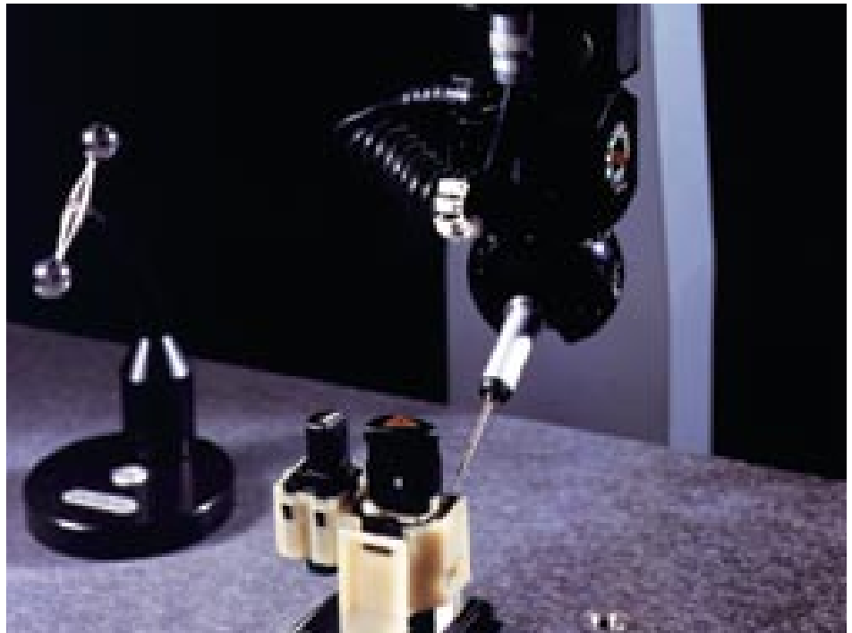
Intricate prototype ignition components can be measured quickly and accurately with the MicroVal PFX.
