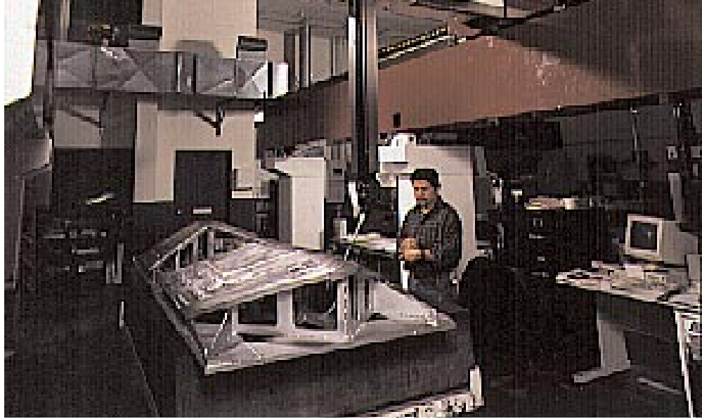
The large size of the DEA DELTA gantry at ADI does not preclude accuracy. It has been certified to a volumetric accuracy of 0.002" to handle dimensional inspection of the most precisely built workpieces.
