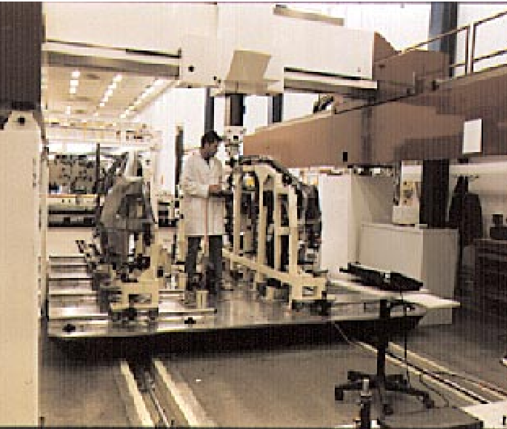
A DEA DELTA gantry-type CMM in SEAT-Martorell's quality lab is used to check the dimensions of a sheet metal sub-assembly destined for use in an auto body. The versatile DELTA has a work area large enough to accommodate a complete car body for dimensional inspection.
