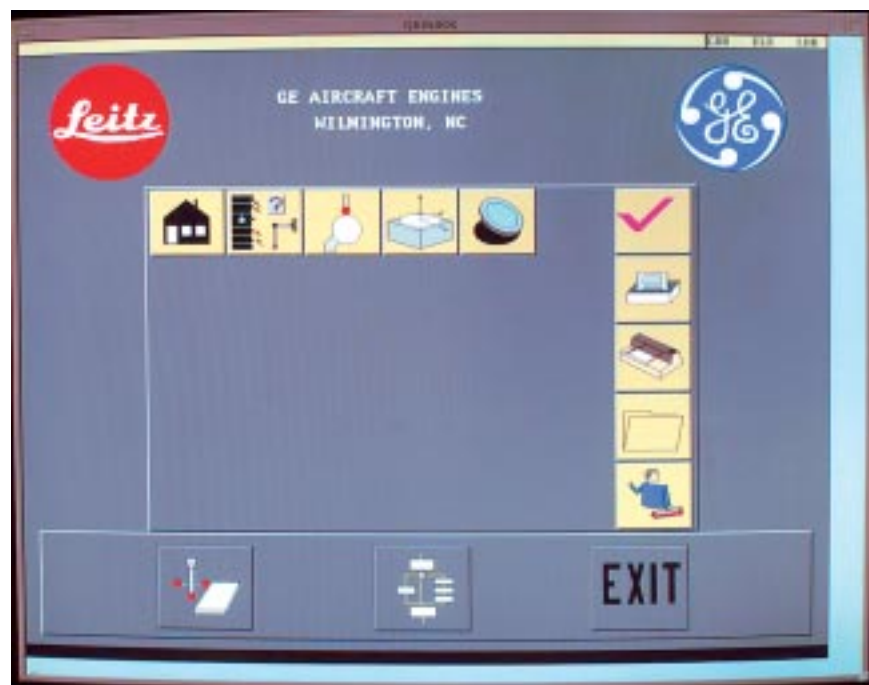
QUINDOS graphic user interface (GUI) leads the operator through powerful inspection routines. From this window, the operator can prepare the SIRIO Shop Floor Gaging Station for measurement operations.
