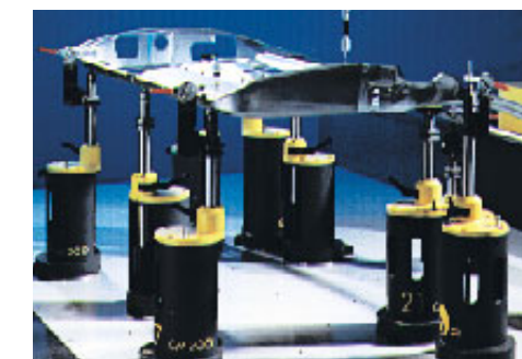
DEA FIVE U-nique Flexible Fixturing System recently purchased by Porsche Stuttgart will eliminate the need for expensive custom workholding fixtures.
