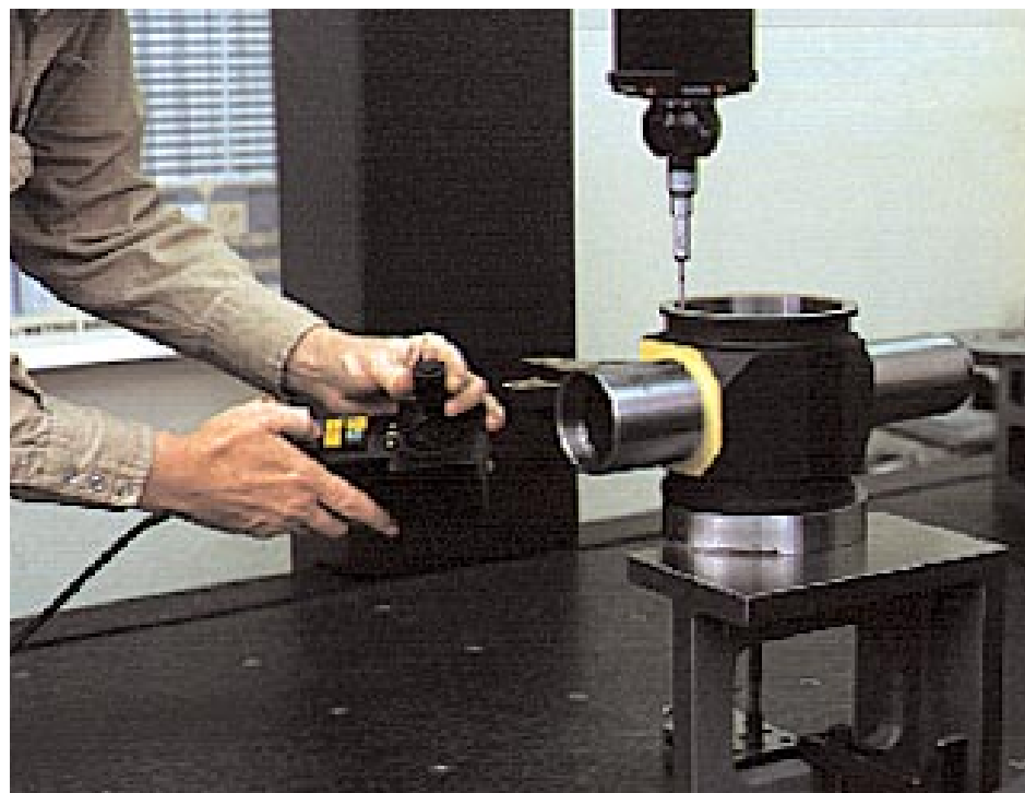
Brown & Sharpe Xcel coordinate measuring machine at B&R Machine and Tool Corp. provides fast, accurate measurement of critical aerospace components. The Xcel's large measuring range can accommodate virtually all of the parts manufactured by B&R.
