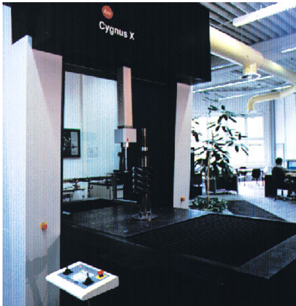
The Leitz Cygnus X combines rugged shop floor measuring speed with laboratory grade accuracy. Caterpillar's Technical Research Center is evaluating this new coordinate measuring machine in a variety of critical dimensional measurement and inspection applications.
