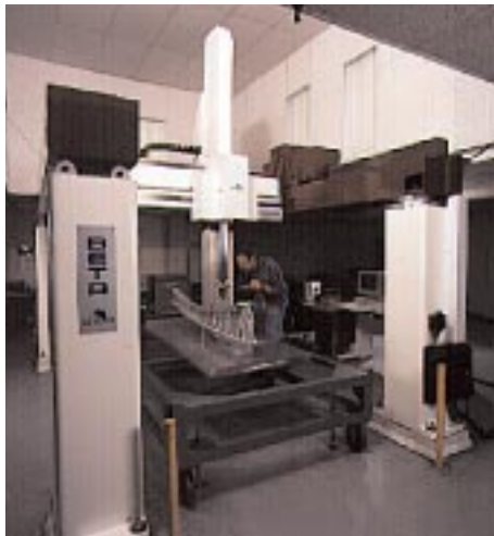
A DEB BETA SP gantry CMM in operation performing a dimensional measurement routine on a large airframe structural component. The BETA is a cost-effective medium-size gantry available in both manual and computer-controlled versions. Its structural design allows the operator to remain close to the part being inspected.
