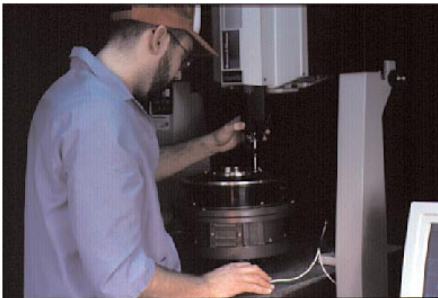
The MicroVal at C.Q. Machining is a versatile manual CMM used primarily to inspect workpieces not having compound angles. It is one of three Brown & Sharpe CMMs at the shop.
