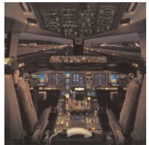
The view from a Boeing 777 cockpit. The 777 is one of the most advanced commercial aircraft in production. Cockpit ergonomics were fine tuned using the Dassault/IBM CATIA design software program to generate human models that repeatedly performed routine and emergency procedures. The CMM determines the fit and finish of virtually every component in the cockpit.
